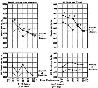
Fig. 17.—Effect of preservative treatment on the strength and stiffness of loblolly-pine stringers treated partially air dry.
